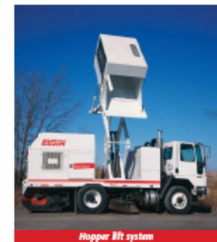
Hopper lift system
