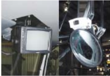
Camera System Camera system, strategically mounted to monitor sweep functions, dumping, and backup movements.
